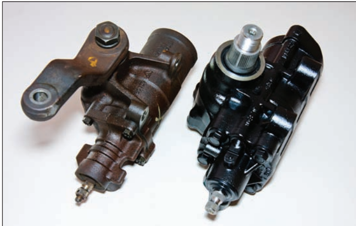
On the left is the original steering gear supplied on new 2003-2008 trucks. The 50% heavier Mopar replacement gear (right), part number 68170214AA, was introduced in 2011.
