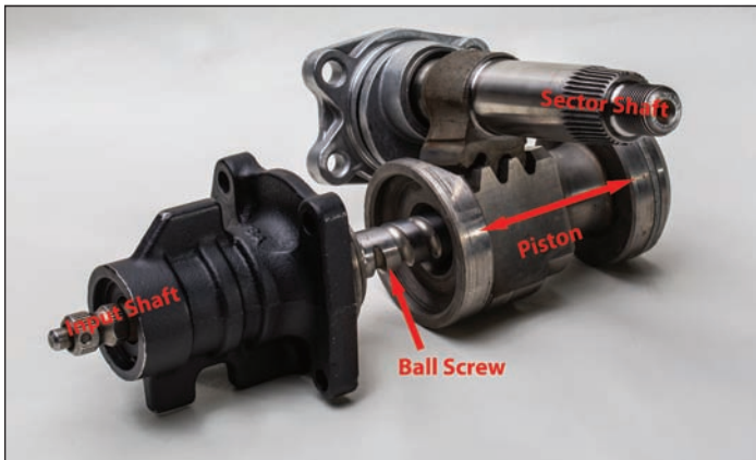
Figure 3. Essential steering gear components, shown without the housing that holds everything together: The input shaft (far left) rotates the ball screw (center), which moves the piston (far right) which rotates the sector shaft (top).
