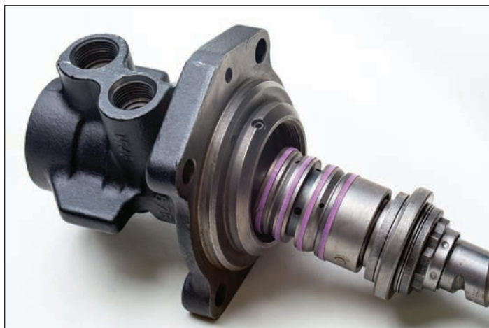
Figure 8. The magic of power steering assist is accomplished by a set of seals, parts, and passageways on the input shaft and mating surfaces of the housing.
